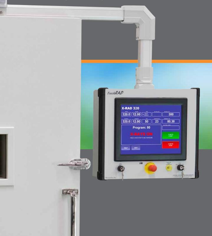
The X-RAD 320 is a self-contained X-ray system for delivering a precise radiation dosage to specimens in a biological or small animal research laboratory.
