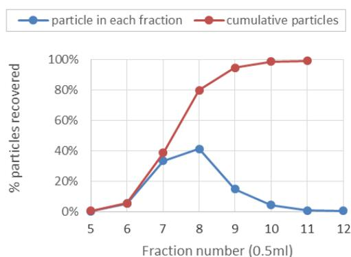
Figure 5 Elution profile for 400 nm polystyrene particles
