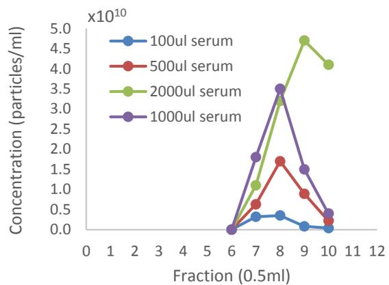
**Figure 3. Vesicle elution profiles for loading of serum from 100 to 2000  $\mu$ L. Loading greater than 500  $\mu$ L extends the elution peak into fractions 9 & 10 where the protein is beginning to elute. High purity is maintained by collecting fractions 7 and 8. Particle concentration is measured in the size range 70-300 nm.**
