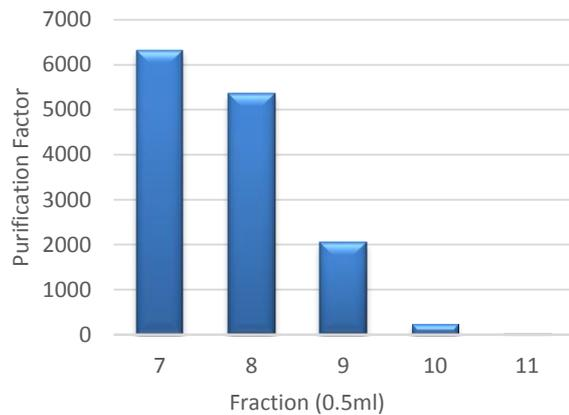
**Figure 1. Typical purification of EVs relative to protein after qEV purification. The purification factor (reduction in ratio of protein after and before SEC isolation) in each fraction is shown. Fraction 7 and 8 were most enriched.**
